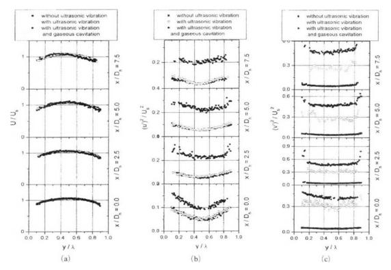
Fig. 6 Axial variations of the stream-wise velocity and the fluctuation intencities due to the ultrasonic vibration and there by induced gaseous cavitation for Re=8,000; (a) stream-wise velocity (b) stream-wise turbulence intensity (c) normal fluctuation intensity
