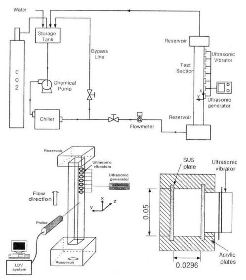
Fig. 3 Schematic diagrams of test loop and test section to investigate the turbulence enhancement by ultrasonically induced CO<sub>2</sub> gaseous cavitation
