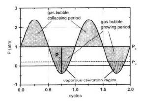
Fig. 1 The mechanisms of vaporous and gaseous cavitation
