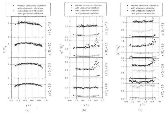
Fig. 4 Axial variations of the stream-wise velocity and fluctuation intensities due to the ultrasonic vibration and there by induced gaseous cavitation for Re=4,000; (a) stream-wise velocity (b) stream-wise fluctuation intensity (c) normal fluctuation intensity
